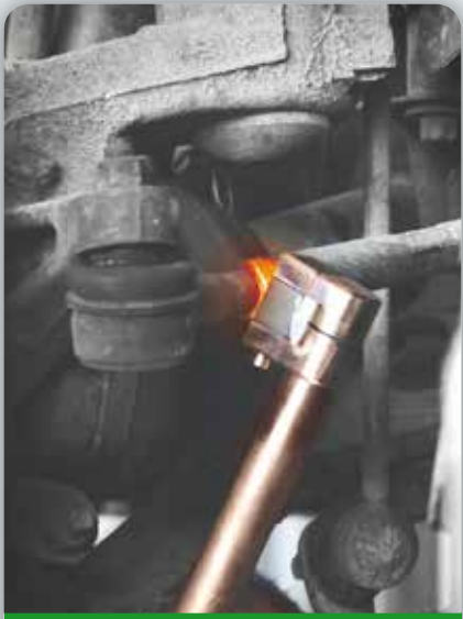
RELEASING CONNECTING RODS ASSEMBLY - DÉGRIPPAGE BIELLETTE DE DIRECTION Small S90 Powerduction 37LG
