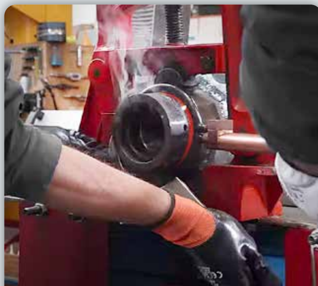
HYDRAULIC CYLINDER MAINTENANCE - MAINTENANCE VÉRINS HYDRAULIQUE Ring inductors Powerduction 220LG
