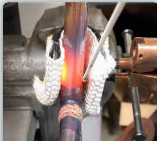
BRAZING COPPER PIPE - BRASAGE TUYAU CUIVRE
