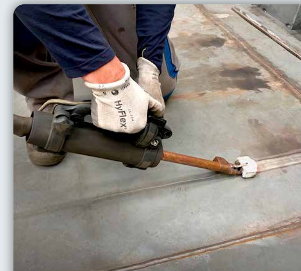
SHIPYARD - HEAT SHRINKING - CONSTRUCTION NAVALE - CHAUDE DE RETRAIT Large L20/B4 Powerduction 220LG
